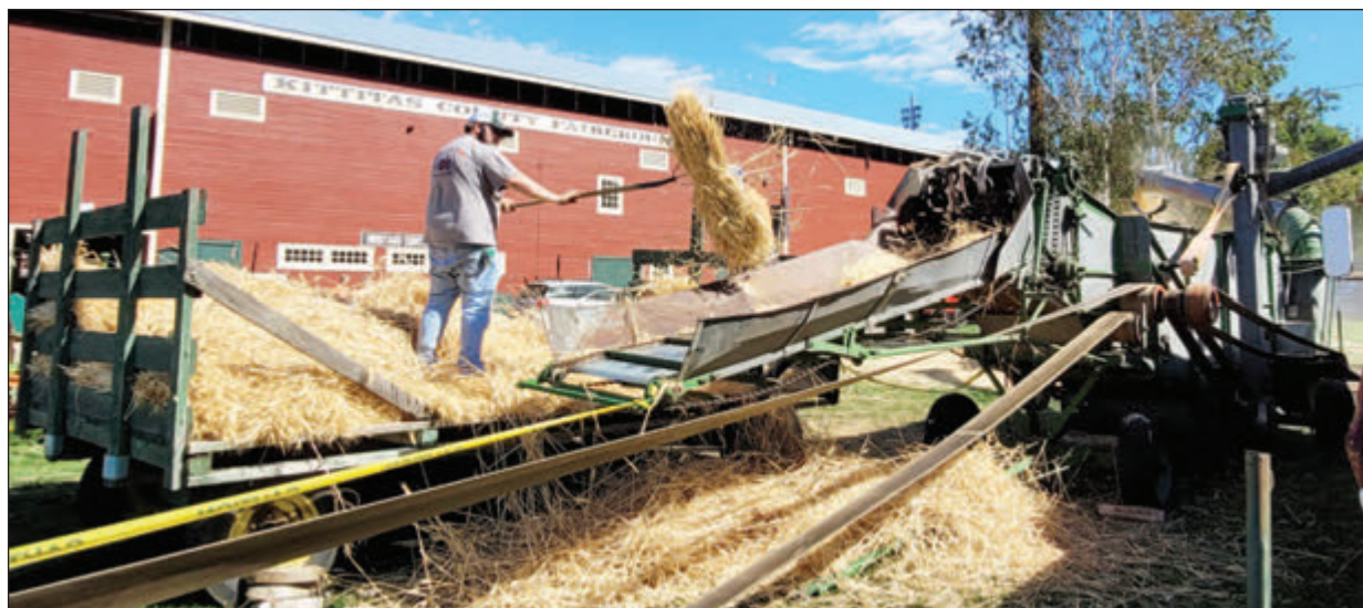
WHEAT IS LOADED into an antique threshing machine which removes the grain from the stalks and husks. This thresher was purchased in 1937 by Hank Stokes from Frank Haagen, a John Deere Dealer in Ellensburg. Hank operated it until 1948 and then it was operated by Vern Stokes into the 1960's. It was acquired by the Kittitas Valley Early Iron Club in 2001.
