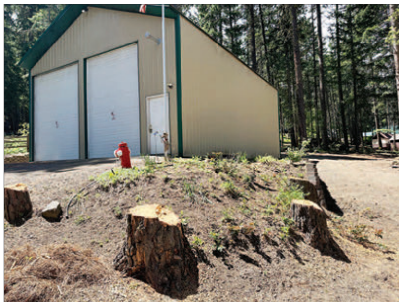
AN EXAMPLE OF trimming back trees and brush to create a defensible space around an outbuilding.
