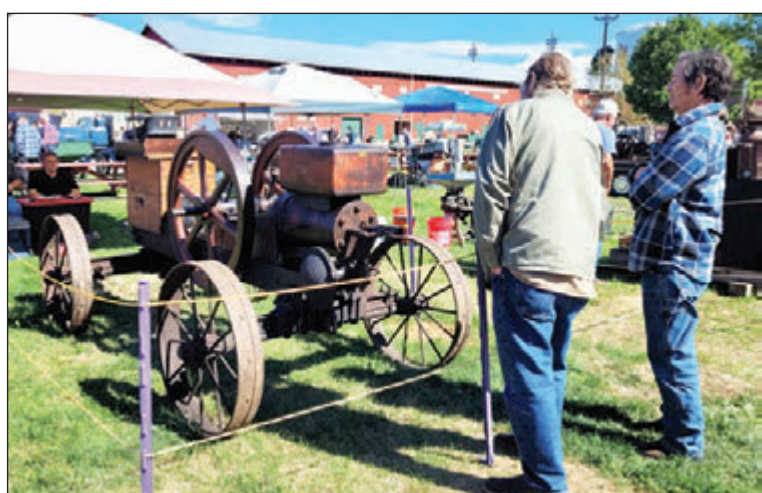
HAY WAS LOADED into this machine and pressed into bales.
