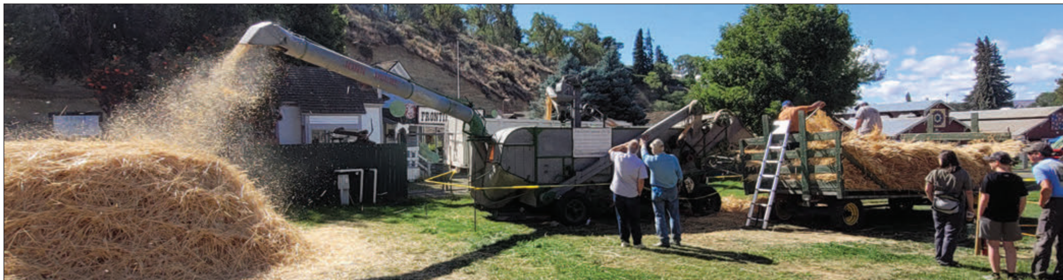
WHEAT IS LOADED into an antique threshing machine which removes the grain from the stalks and husks. This thresher was purchased in 1937 by Hank Stokes from Frank Haagen, a John Deere Dealer in Ellensburg. Hank operated it until 1948 and then it was operated by Vern Stokes into the 1960's. It was acquired by the Kittitas Valley Early Iron Club in 2001.
